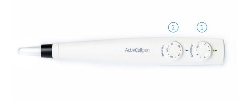
The two rotary switches allow an adjustment of the energy at the tip of the electrodes that is converted into cold atmospheric plasma.
